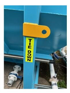
DO NOT STRAP OVER UNIT AS THIS CAN DAMAGE THE COLLAPSIBLE PLATFORM
