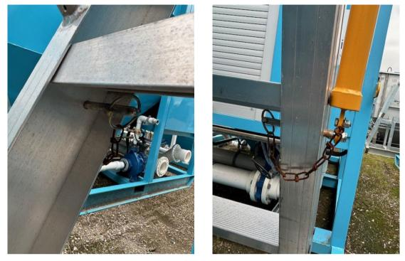
2. Remove locking bolt from the ladder and push the bar up, this will erect the handrail
